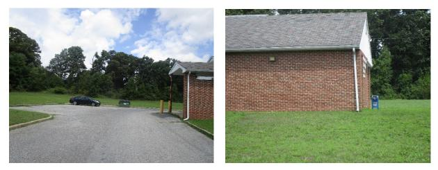
A strip of parking lot on the east side of the building can be replaced with pervious pavement to capture and infiltrate stormwater runoff from the parking lot. A rain garden can be installed on the south side of the building to capture, treat, and infiltrate rooftop runoff. A preliminary soil assessment suggests that the soils have suitable drainage characteristics for green infrastructure.
