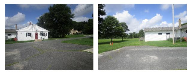
A rain garden can be installed at the southeast corner of the building to capture, treat, and infiltrate stormwater runoff from the rooftop. A preliminary soil assessment suggests that more soil testing would be required before determining the soil's suitability for green infrastructure.
